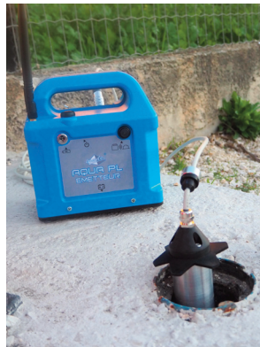
Water column injection
